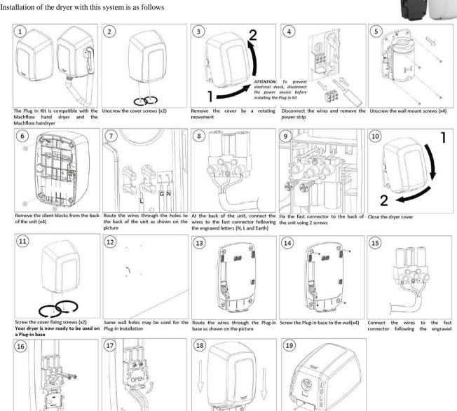
Mount the dryer over the Plug-in base
